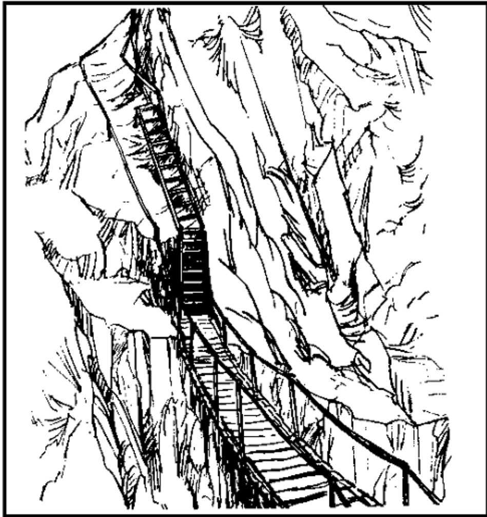
Figure 2-2. Suspended Walkway and Standoff Ladders.
